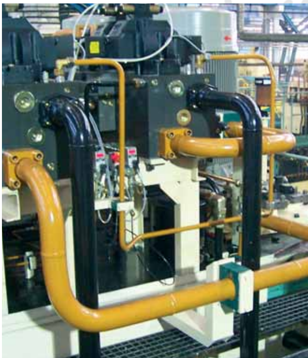
Hydraulika lisu 800 t ■ Hydraulics of the press 800 t
